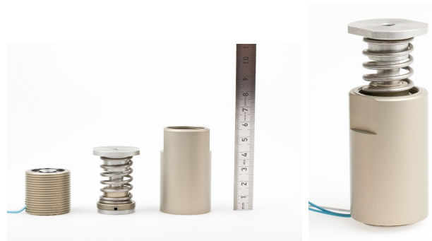
Fig. 3. The Grasp Perturbator; from left to right: electromagnet, moving part, rigid part, whole.
