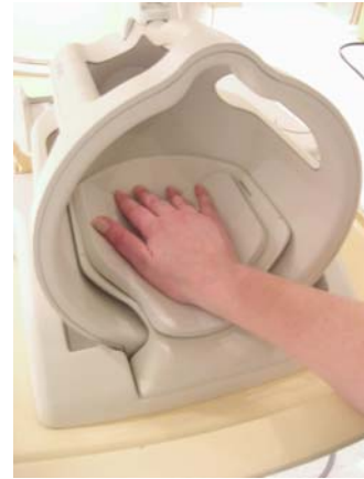
Fig. 2. Hand inside a Philips SENSE head coil, which improves image quality on small body structures. The hand and the shown coil are inserted into the large MRI tube during the recording of the images.
